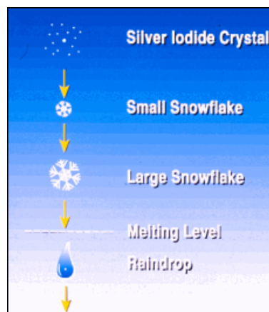
Figure 3a Cloud Seeding Process
