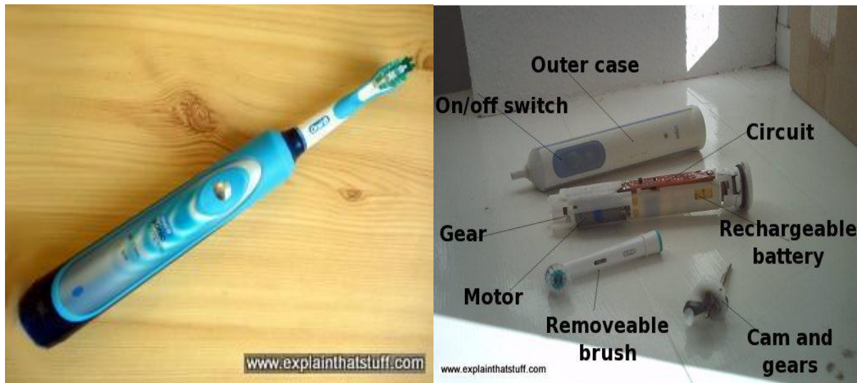
Figure 3: The electric rotation-oscillation toothbrush and different parts that compose it
