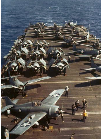
Figure 5. The Grumman F4F Wildcats on the left side of the picture demonstrated the use of wing-folding mechanism to save space on an aircraft carrier.
