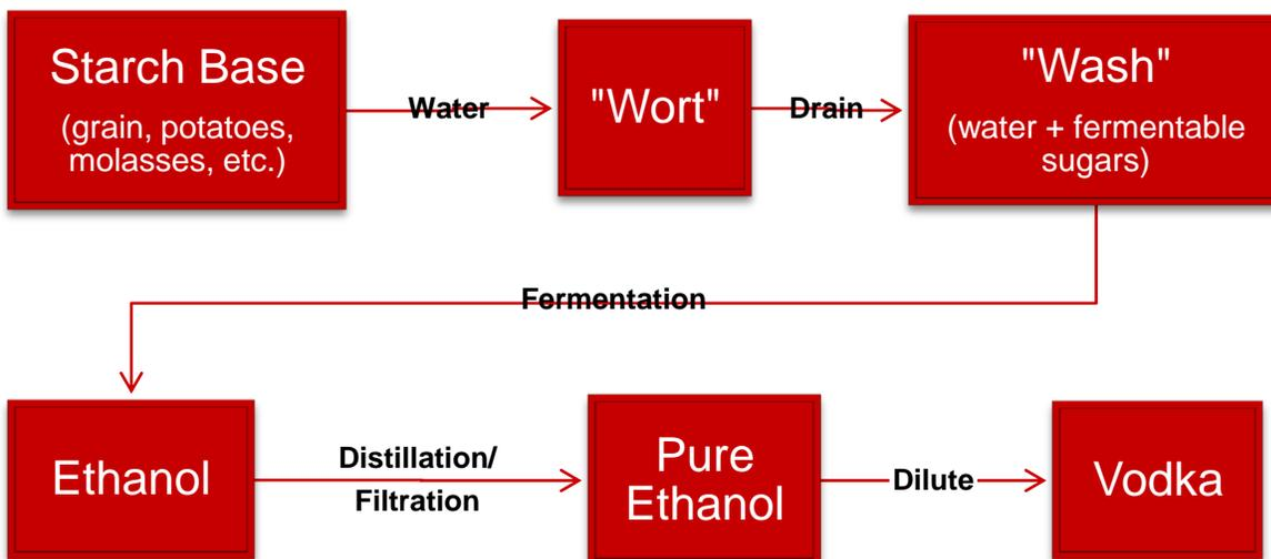
Figure 1. Steps in the vodka manufacturing process.
