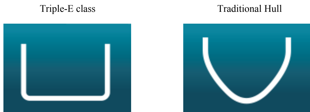
Figure 1. Triple-E hull shape compared with traditional container ship hull shape.
