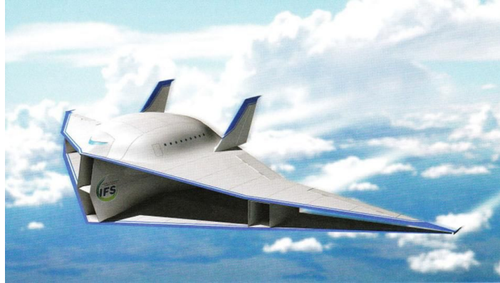
Figure 6. A biplane with two layers of wing on each side of the aircraft
