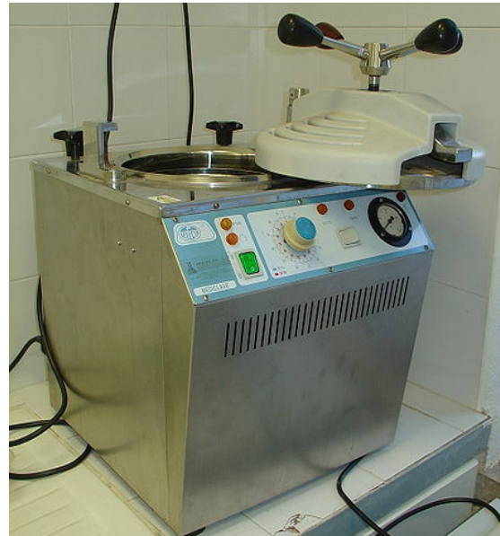
Figure 1. Autoclave Small, commercial autoclave with top closure. Image Source: Wikimedia Commons
